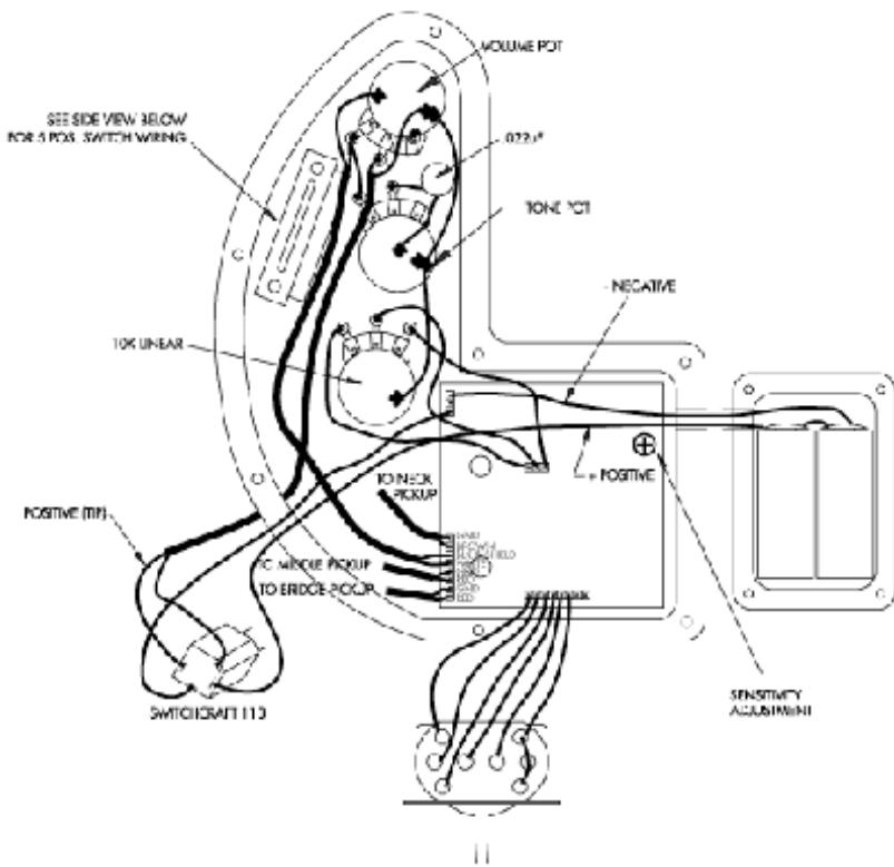
**7. Five Position Pickup Selector:** When the Infinity Sustainer is OFF, this operates as follows:
